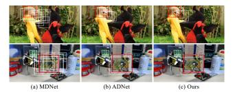
Figure 1: The different strategies of three tracking algorithms. (a) MDNet (Nam and Han 2016): classify with random sampling; (b) ADNet (Yun et al. 2017): iterative search with a series of discrete actions; and (c) our tracker: DRLbased hierarchical search with less continuous actions.
