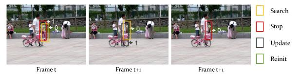
Figure 3: An illustrative example of the tracking mode switch controlled by the policy agent: 1) at frame t, the object is readily located by one *search* step; 2) at frame t + 1, firstly, a *search* step tends to a distractor nearby, than the policy agent realizes this and takes an *update* action to conduct expert demonstration; 3) the current tracking result is updated by the expert tracker.
