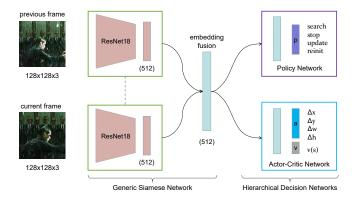
Figure 2: The overview of the proposed tracking framework. PACNet is constituted by a shared feature extractor for observation, a policy network for mode switch and an actorcritic network with an LSTM layer to perform searching.
