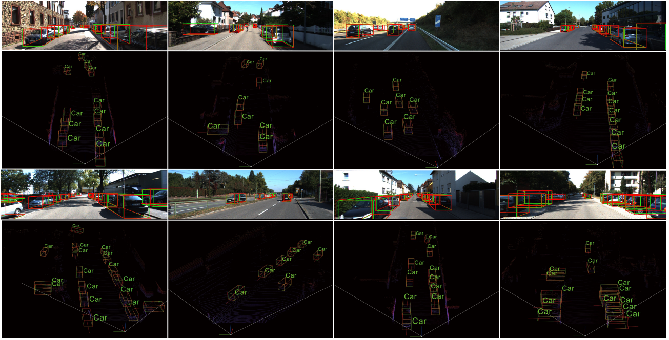
Figure 5: Qualitative results of PC-RGNN on the KITTI val split (best viewed with zoom-in). For each sample, the upper part is the image and the lower part is a representative view of the corresponding point cloud. The red boxes indicate the predicted results while the green ones denote the ground-truths.
