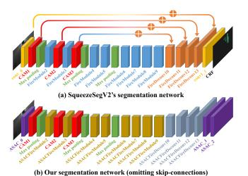
Figure 3: Our segmentation network vs. SqueezeSegV2 (Wu et al. 2019). We replace all standard convolution (conv) and the final conditional random field (CRF) with aligned spatially-adaptive convolution (ASAC). We replace all batch normalization after each conv with instance normalization.
