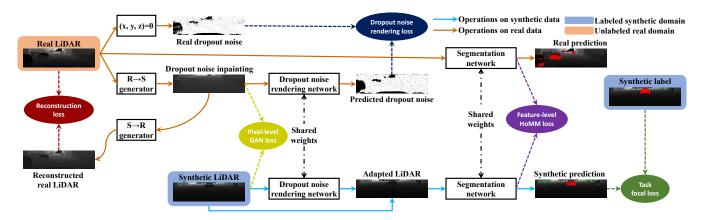
Figure 2: The proposed SRDA framework ePointDA for LiDAR point cloud segmentation. The colored dashed arrows correspond to different losses. For clarity the real-to-simulation cycle is omitted. See Figure 3 for detailed segmentation network.
