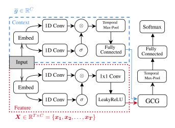
Figure 3: Our new proposed architecture with global channel gating (GCG). The blue thick dashed sub-network shows the context extractor, which is used to suppress information found from the Feature extraction sub-network (red, thinly dashed sub-network).
