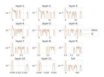
Figure 1: Eigenspectra of  $\{\text{Hess}_l\}_{l=1}^L$  and  $\{G_l\}_{l=1}^L$  on VGG11+BatchNormalization model trained on CIFAR-10 (Best viewed in color). Note that where the graph of the Hessian is not visible, the spectra of Hessian and G overlap completely. The last subplot "full" refers to eigenspectra of the Hess and G of the entire network;
