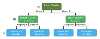
Figure 2: A basic NDT architecture. Given an input: (1) Each node determines which of two groups of class labels the input belongs to; (2) Once identified, input is passed to the next respective model in the tree; (3) Finally, at the leaf nodes, if the predicted subgroup only contains a single label, a final classification is output. The predicted class is determined by the path of the input through the NDT.
