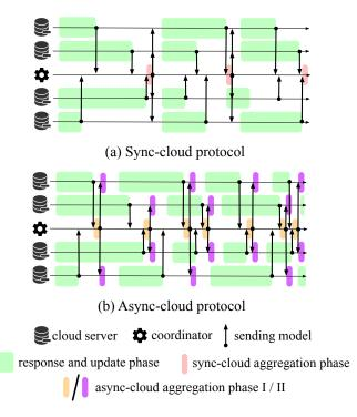
Figure 2: Protocols under Sync-/Async-cloud architectures.
