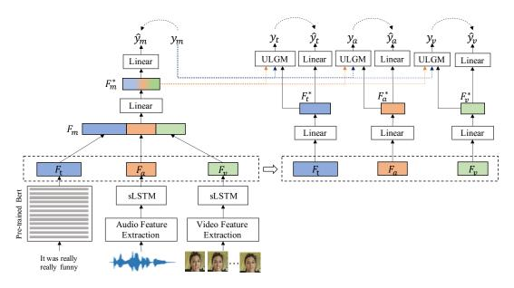
Figure 2: The overall architecture of Self-MM. The  $\hat{y}_m$ ,  $\hat{y}_t$ ,  $\hat{y}_a$ , and  $\hat{y}_v$  are the predictive outputs of the multimodal task and the three unimodal tasks, respectively. The  $y_m$  is the multimodal annotation by human. The  $y_t$ ,  $y_a$ , and  $y_v$  are the unimodal supervision generated by the self-supervised strategy. Finally,  $\hat{y}_m$  is used as the sentiment output.
