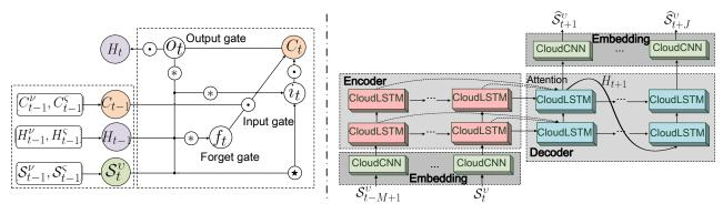
Figure 3: The inner structure of the CloudLSTM cell (left) and the overall Seq2seq CloudLSTM architecture (right). We denote by  $(\cdot)^{\nu}$  and  $(\cdot)^{\varsigma}$  the value and coordinate features of each input, while these features are unified for gates.
