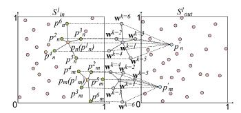
Figure 2: DConv operation with a single input channel and  $\mathcal{K}=6$  neighbors. For every  $p\in\mathcal{S}_{in}^1$ , DConv weights its  $\mathcal{K}$  neighboring set  $\mathcal{Q}_n^{\mathcal{K}}=\{p_n^1,\cdots,p_n^6\}$  to produce values and coordinate features for  $p_n'\in\mathcal{S}_{out}^1$ . Here, each  $\mathbf{w}^k$  is a set of weights w with index k (i.e., k-th nearest neighbor) in Eq. 2, shared across different p.
