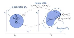
Figure 1: The conservative reachset  $\mathcal{B}_j$  at time  $t_j$  computed using Lagrangian reachability and global optimization, for a Neural ODE starting from the ball  $\mathcal{B}_0$  at time  $t_0$ .
