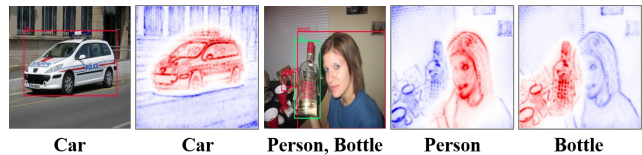
Figure 1: Relative Sectional Propagation (RSP) aims to fully decompose the network predictions with taking advantages of i) strong objectness, ii) class-discriminateness, and iii) detailed descriptions of neuron activations.
