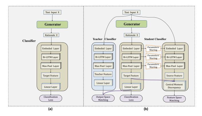
Figure 1: Comparison of (a) the baseline RNP framework, and (b) our proposed DMR framework. We run the classifier on the full input text for feature matching, and also train a student classifier for output matching.
