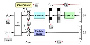
Figure 2: Architecture of InfoCal: the grey round boxes stand for the losses, and the red arrows indicate the data required for the calculation of losses. FFL is an abbreviation for feed-forward layer.
