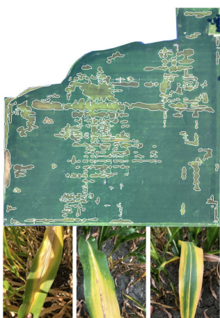
Figure 1: Nutrient Deficiency Stress appear brighter green in this aerial image which have been annotated with polygons(top). By alerting farmers to regions of the field experiencing NDS, further ground-level inspection can reveal what type of nutrient deficiency exists so the best management decisions can be made. Ground-level images of interveinal (bottom left), nitrogen (bottom middle), and potassium (bottom right) stress.
