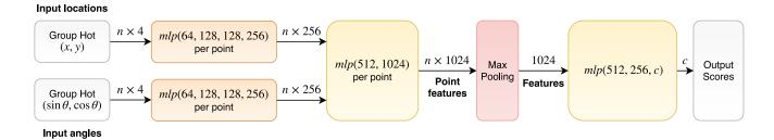
Figure 3: Network architecture, consisting of two pathlines: location and angle.
