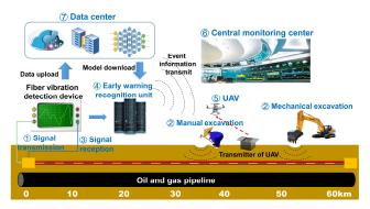
Figure 1. Structure of oil and gas PSEW system
