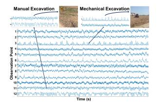
Figure 5. Waveforms of signals collected at a China National Petroleum Corporation pipeline
