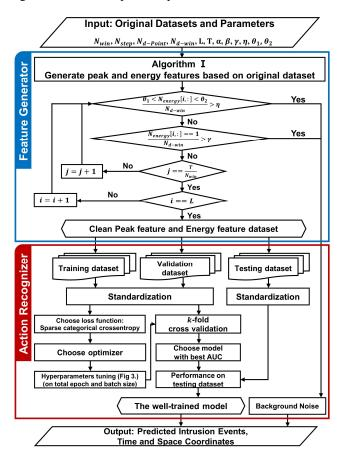
Figure 4. Collaborative workflow of the feature generator and action recognizer
