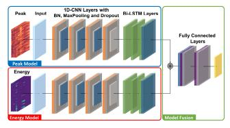
Figure 3. Action recognizer model. Orange is the Conv1D layer, dark grey is batch normalization, light grey is max-pooling, blue is dropout, green is the Bi-LSTM layer, and purple is the fully connected layer. The standardized peak and standardized energy features were expressed by heat maps and contour maps respectively.
