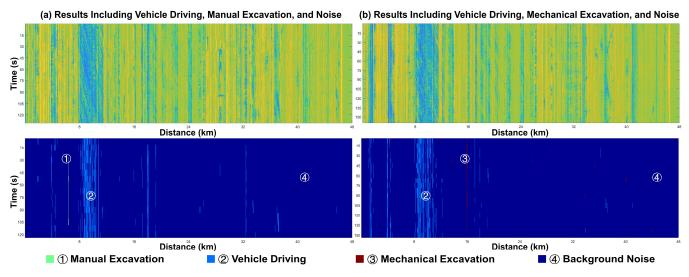
Figure 10. Heat maps comparing peak features and identification results from a real 48-km pipeline. The upper part of each graph shows the peak features of intrusion events, the lower half shows the identification results of intrusion events. (a) We can see that manual excavation events appeared at approximately 6 km and lasted nearly 90 s. (b) We can see that mechanical excavation events appeared at 16 km and lasted about 140 s. There were also continuous vehicle driving events at 8 to 10 km.
