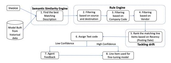
Figure 2: Architecture of proposed system involving Semantic Similarity Engine, Rule Engine, module for tackling Drift, Feedback Mechanism and Online training
