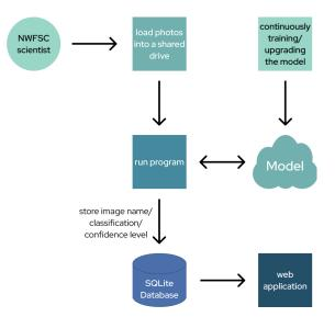
Figure 2: Overall system design
