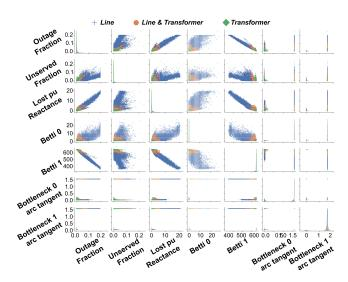
Figure 6: Scatterplot of the relationship between dependent variable (fraction of load not served, shown in the second row and second column) and independent variables in the contingency dataset under the electrical-distance weighting scheme.
