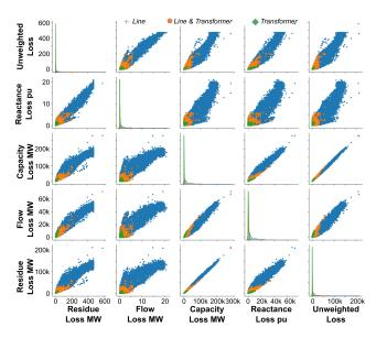
Figure 4: Scatterplot matrix of the relationship between the total weights of outaged components for the unweighted and four weighting schemes.
