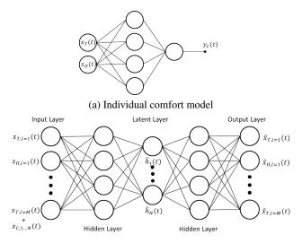
(b) The thermal sensor model and the thermal set point model shown in the autoencoding framework.
