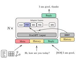
Figure 1: Adapter-Bot high-level architecture.
