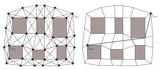
Figure 1: NavMesh: Shortest Path Formed by Graph Edges (left) vs. Truly Shortest Path (right)
