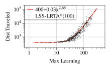
Figure 10: Solution cost versus max learning for any state when solving a problem instance using LSS-LRTA\* with lookahead depths of 1, 10 and 100.
