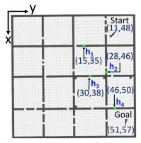
Figure 1: Robot navigation between rooms with doors whose status (open/closed) is unknown.
