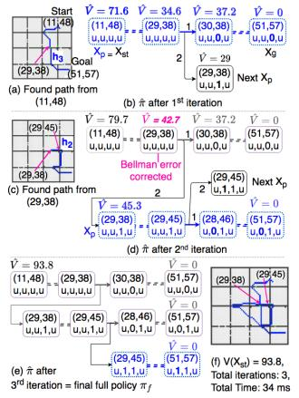
Figure 3: FAST-PPCP operation in [**Ex.**]. Numbers 1 and 2 near a stochastic transition (solid arrows in a partial policy) indicate transition costs. Outcomes of deterministic *move* actions have been omitted (visualized as dotted lines).
