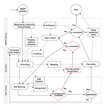
Figure 1: Scheme of DPLL(MAPF) consisting of SMT-CBS scheme and consistency checking (marked red) against MAPF rules.
