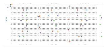
Figure 2: A  $32 \times 75$  sized warehouse, densely packed with 876 shelves (in gray) and operated by 54 agents (coloured dots). Experiment video: https://bit.ly/3aMIomO
