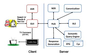
Figure 2: Architecture overview. The Hub invokes the spokes in a clock-wise manner starting with NER.
