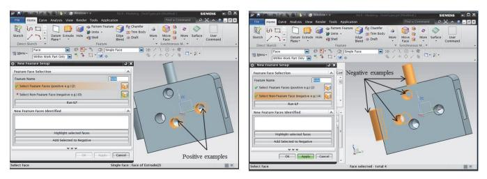
Figure 5. Selecting Examples for Blind Holes with Conical Bottom - Selections Displayed in Orange and with Arrows. (a) Positive Examples. (b) Negative Examples.
