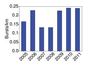
Figure 1: Bursts per km of pipe length in each year. The data is shown for large diameter pipes.
