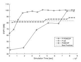
Figure 2: Convergence of P-POMCDP, POMCDP, and P-GA. For P-POMCDP and POMCDP each point in the graph shows the expected NPV of the policy at the corresponding simulation time. For P-GA each point shows the expected NPV of the best solution found so far. Best practices represent the best FDP suggested by subject matter experts.
