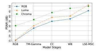
Figure 3: Ablation study for the proposed techniques. We compare, in terms of PSNR, the intermediate steps  $x_i$  with the original RAW image at both RGB and YUV (luminance Y, chrominance UV) colour domains. Results show a monotonic PSNR evolution at RGB domain, meaning that after each transformation the RGB moves "closer" to the RAW image.
