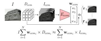
Figure 2: Dictionary-based Color Space Transformation. During training,  $D_{ccm}$  and  $E_{ccm}$  are learned together and generate a single output. At inference time, dictionary augmentations are used to generate k samples from a single RGB input. The  $\mathbf{r}_k$  represent the random perturbations added to  $\mathbf{w}_{ccm}$ .
