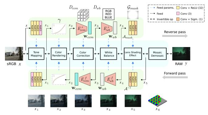
Figure 1: A visualization of our proposed model using as backbone (blue) the classical ISP operations described in Section 2, and additional learning component (green) described in Section 3. RAW images are visualized through bilinear demosaicing.
