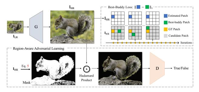
Figure 2: The framework of our Beby-GAN. The best-buddy loss allows the estimated HR patches to be supervised in a dynamic way during training. The region-aware adversarial learning is proposed to make the discriminator focus on rich-texture areas.
