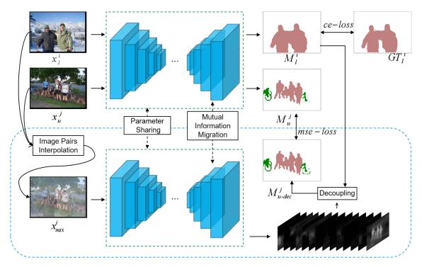
Figure 2: Overview of our proposed semi-supervised segmentation approach. GuidedMix-Net follows the basic architecture of U-Net, consisting of an encoder-decoder architecture. The main decoder is constructed by ResNet, while the decoder is incorporated by our MITrans modules.
