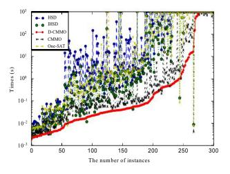
Figure 4: Runtime for the ISCAS-85 benchmark circuit using S-A-0 fault model.
