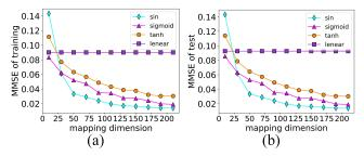
Figure 1: The effects of mapping dimension and activation function to the model inference accuracy. (a) MMSE of the training set. (b) MMSE of the test set.
