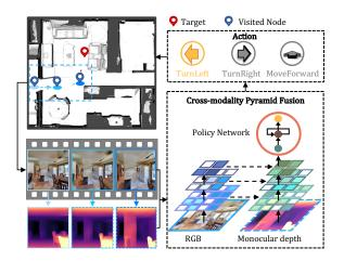
Figure 1: Illustration of Geo-Nav framework. An agent predicts monocular depth by Self-supervised Depth Estimation network (SDE). The agent applies Cross-modality Pyramid Fusion module (CPF) to merge features from the RGB image and estimated depth map into an informative visual representation. Then, the agent produces a navigation policy and selects an action, *e.g.*, TurnLeft. The red point represents the target position, and visited nodes are highlighted by blue points in one episode.
