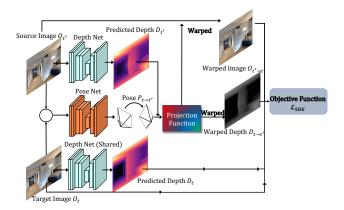
Figure 3: Illustration of Self-supervised Depth Estimation network (SDE).
