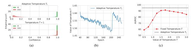
Figure 4: Ablation study on the adaptive temperature  $T_t$ . (a): Empirical p.d.f. of the output confidence of the samples in U with  $T_t$  (upper part) and T = 1 (lower part). (b): The values of  $T_t$  during training. (c) Detection results on U with different T.
