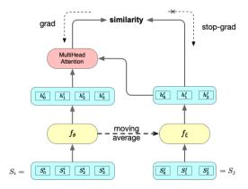
Figure 2: The contrastive objective.  $S_i$  and  $S_j$  are two sequences to contrast,  $f_{\theta}$  and  $f_{\xi}$  have the same architecture,  $\theta$  in  $f_{\theta}$  is updated by gradient decent while  $\xi$  in  $f_{\xi}$  is the moving average of  $\theta$ .
