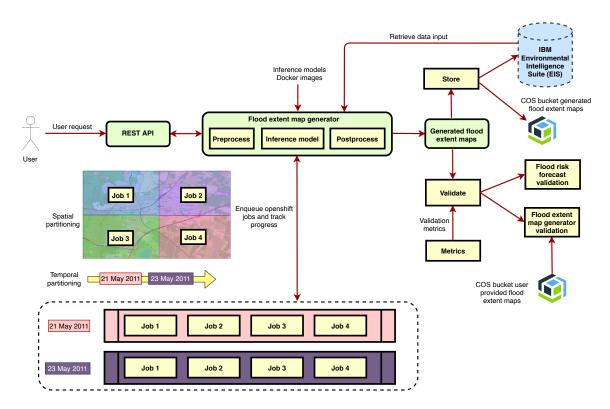
Figure 1: The high-level architecture for the REST API service for inference with temporal and spatial partitioning.
