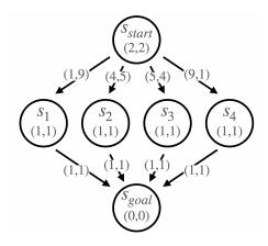
Figure 3: An example problem instance whose Paretooptimal frontier consists of four paths. The pair of numbers inside each state is its h-value. The pair of numbers annotating each edge is its cost.
