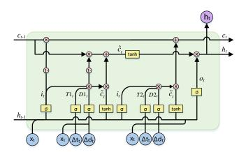
Figure 3: A variant of STGN using coupled input and forget gates.
