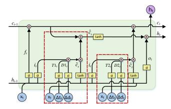
Figure 2: STGN has two time gates and two distance gates, i.e.,  $T1_t$ ,  $T2_t$ ,  $D1_t$  and  $D2_t$ .  $T1_t$  and  $D1_t$  are designed to model time and distance intervals for short-term interests while  $T2_t$  and  $D2_t$  are to model time and distance intervals for long-term interest.
