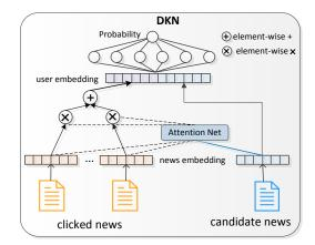
Figure 1: Simple visualization of DKN model.
