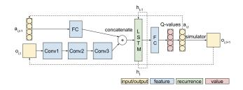
Figure 3: One time slice of ADRQN. Inputs are  $a_{i,t-1}$  and  $o_{i,t}$ , outputs are  $a_{i,t}$  and  $o_{i,t+1}$ . FC stands for fully connected layer. Conv stands for convolutional layers. Output of LSTM layer  $h_t$  will be input into LSTM in the next time slice. Actual hyper parameters vary on different problems.
