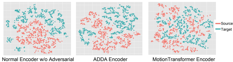
Figure 5: Visualization of extracted representations in the source and target domains. It can be seen that the MotionTransformer leads to a more consistent latent representation compared with the disjoint representations of the normal encoder and the ADDA encoder.
