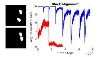
Figure 4: Left: block alignment problem. Top left: two blocks are placed randomly. Bottom left: the agent must pick up one block and place it roughly in alignment with the second. Right: learning curves for simulated blocks world domain. Blue: DIM with hierarchical value function only in last two curriculum steps. Red: DQN baseline.
