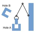
Figure 1: A policy for inserting a peg into Hole A learned using deictic image mapping generalizes to Hole B without any additional training.
