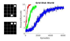
Figure 2: Left: the GRID-DISK domain. Disks are initially placed on a grid randomly (top left). The agent must pick one disk and place it adjacent to another (bottom left). Right: learning curves averaged over 10 runs for DQN applied to GRID-DISK for a  $3 \times 3$  grid (red), a  $4 \times 4$  grid (green), and a  $5 \times 5$  grid (blue).
