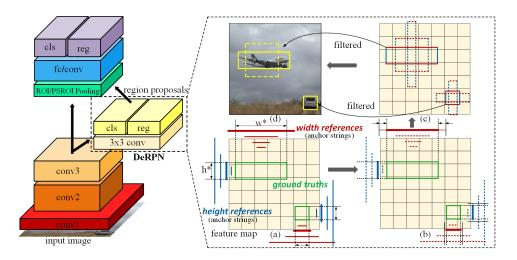
Figure 2: DeRPN network and pipeline. (a) Object widths and heights are independently matched with anchor strings. Bold lines represent well-matched anchor strings. This step is employed during the training phase. (b) We apply classification and regression on anchor strings. Dashed lines are anchor strings of low probability. (c) Predicted width and height segments are combined to compose bounding boxes. (d) We filter bounding boxes by probability and NMS to generate region proposals.
