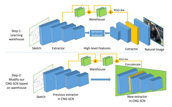
Figure 3: The illustration of learning the latent Sketch-to-Image warehouse. The feature extractors are components of CGN-SCN. The warehouse networks are stacks of convolutional layers and all of them do not change the size of input. In the first step, we train the warehouse network based on the feature maps of sketches and natural images. Then we integrate the warehouse network into the CNG-SCN to improve the performance in the second step.
