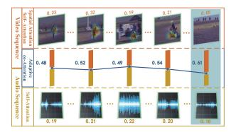
Figure 1: The diagram of audio-visual sequence of temporal inconsistency. At the last time segment, the event only occurs in audio but does not occur in the video. Our network can cope with such challenge by automatically learning to pay higher attention on specific visual regions, specific time segments and specific modality where the event occurs.
