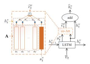
Figure 4: A illustration of cross-modal adaptive co-attention module generating visual modality sentinel  $\beta_t^v$  and the new context vector  $\hat{c}_t^v$ .
