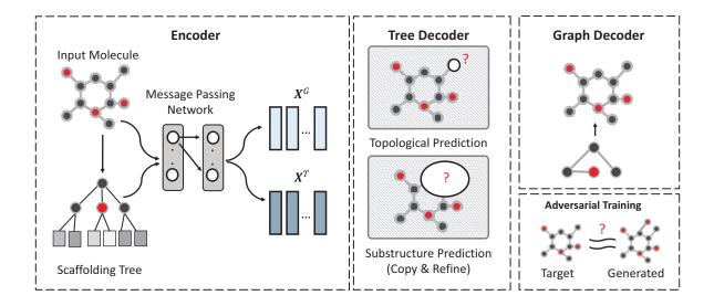
Figure 1: Pipeline for Graph-to-Graph Model. Encoder include both graph and scaffolding tree levels. Decoding mainly split two parts scaffolding tree decoder and graph decoder. scaffolding tree decoder generate molecule in greedy manner using Depth First Search with topological and substructure prediction on each node. To assemble the node of scaffolding tree into the molecule, graph decoder enumerates all possible combinations.
