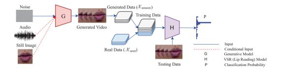
Figure 1: Overall pipeline demonstrated with the generator G as the TC-GAN architecture
